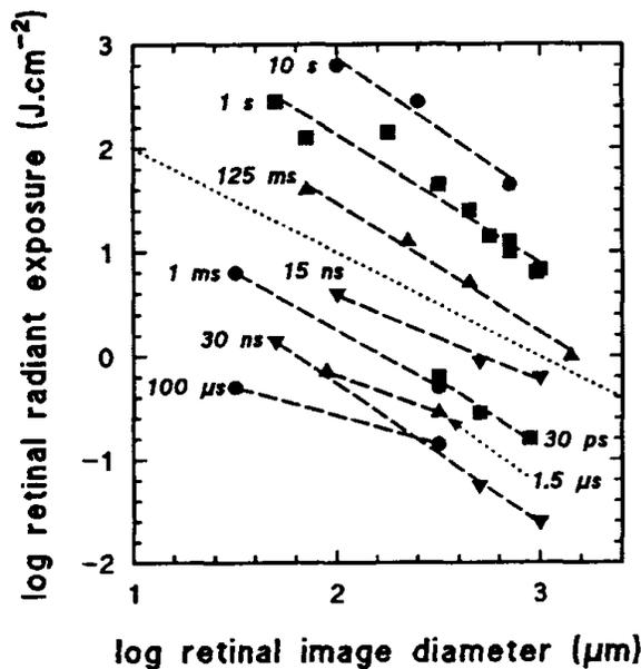
**Figure 116-17.** Log retinal radiant exposure for threshold lesions plotted against log of the diameter of the retinal image for various exposure times. The dashed lines are least squares fits through each set of data, and the dotted line has a slope of - 1. (Data from Sliney.<sup>22</sup>)
