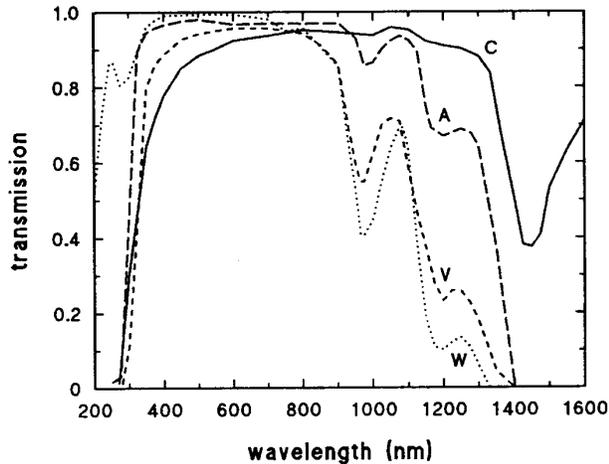
**Figure 116-3.** Spectral transmission curves of rhesus monkey ocular media. C, Cornea (path length = 0.55 mm),. A aqueous (path length 2.86 mm); V, vitreous (path length = 11.55 mm); and, for comparison, the dotted curve, W, of distilled water (path length = 18.5 mm). (Data from Maher.<sup>11</sup>)
