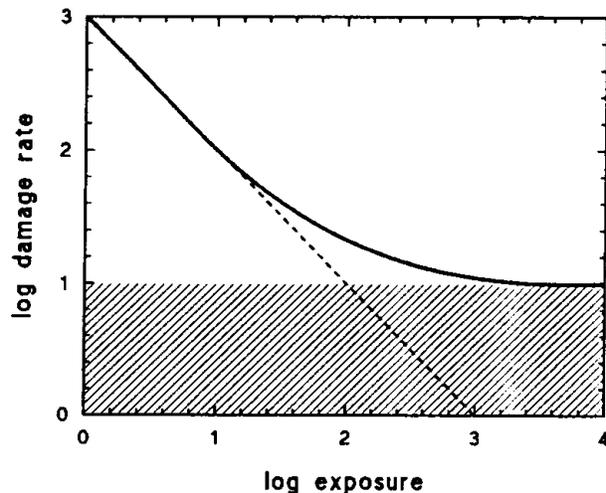
**Figure 116-15.** Damage rate (or irradiance) plotted against duration of exposure for photochemical retinal damage (both axes in arbitrary units). The shaded area represents the area where repair processes exceed the rate of degradation, the dashed line shows the reciprocity relation of slope - 1, and the solid line the practical division between damage and no damage.
