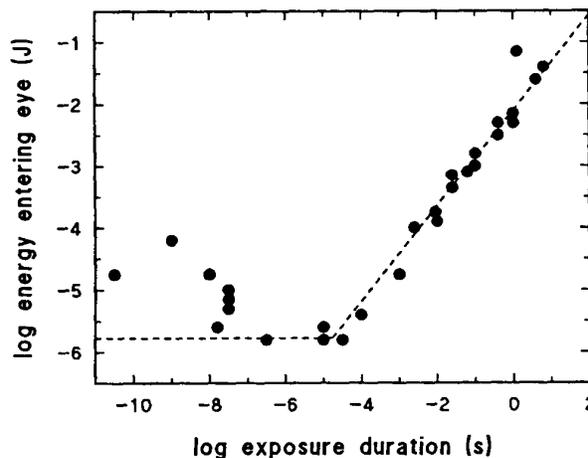
**Figure 116-19.** Log of the energy entering the eye that causes threshold thermal damage plotted against log exposure duration. The line has a slope of 0.75 and is a by-eye fit. (Data from Sliney.<sup>22</sup>)
