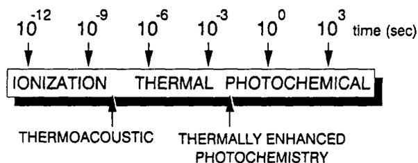
**Figure 116-8.** The mechanisms for light-induced retinal damage related to exposure duration.
